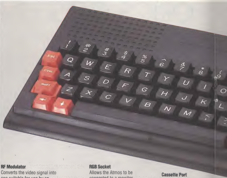
Oric-1 The Atmos is an updated version of the Oric-1. It uses the same circuit board but has a different ROM chip that holds an improved version of BASIC. These changes are sufficient to make the Atmos a far better machine. Owners of the Oric-1 can pay £60 to upgrade to the Atmos standard. However, much of the Oric's software will not work on the Atmos, so users may find themselves unable to use their favourite programs
